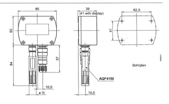
Dimensioning without (with) LCD-display Dimensions in mm
